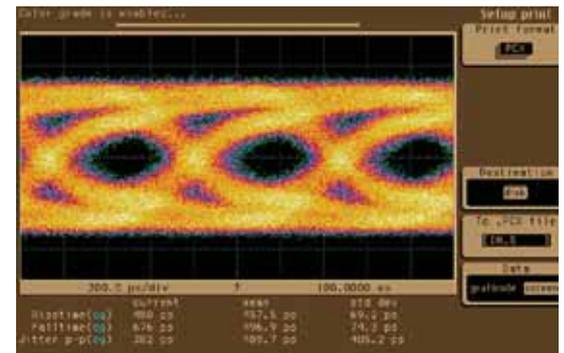
Figure 3. An example of a poor eye test
