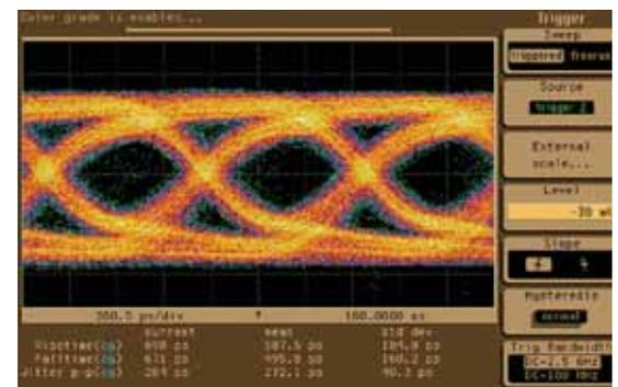
Figure 4. This eye test is better than Figure 3, but it still contains too much noise and jitter.
