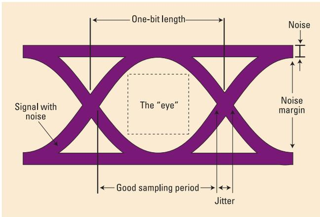
Figure 1. Eye test components
